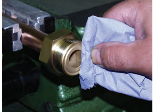
8. Before assembling clean the DILO tongue and groove part
